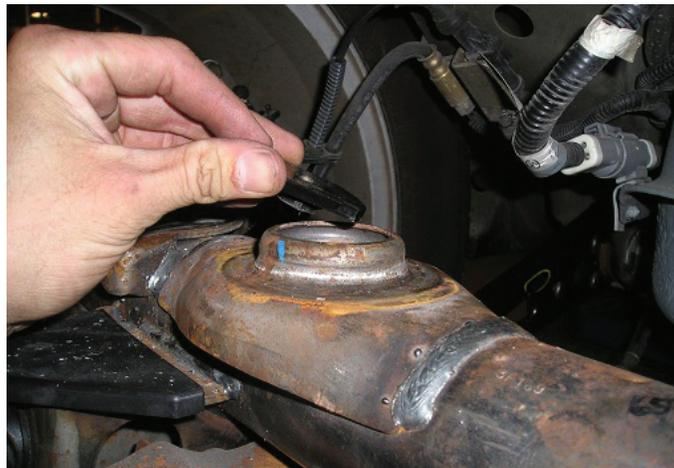
4. Place the plastic spacer (J) over the lower coil spring perch (Fig. 9).
